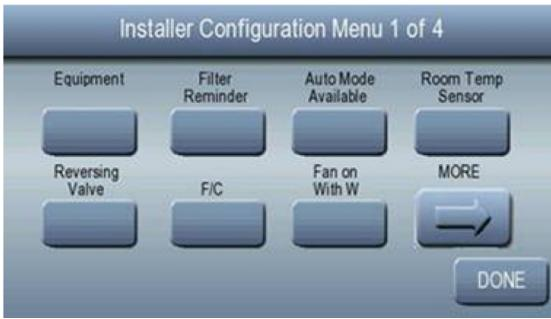
**NOTE:** The **INSTALL / SERVICE** menu will automatically exit after 90 seconds of no activity.
