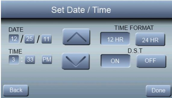
Under date, you can select the month, day, or year buttons; then use the ▲ and ▼ to select the appropriate date. . Under time, you can select the hour, minute, and am/pm; then use the ▲ and ▼ to select the appropriate time. You also have the option of selecting between a **12 HR** or **24 HR** clock format. Finally, you can choose whether you observe day light savings time by pressing the **ON** or **OFF** button. Press
